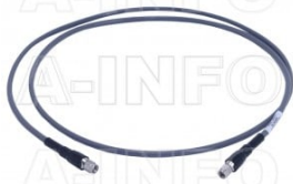
SM-SM-A080-1500 Flexible Cable Assembly 1500mm DC- 26.5GHz SMA Male to SMA Male
